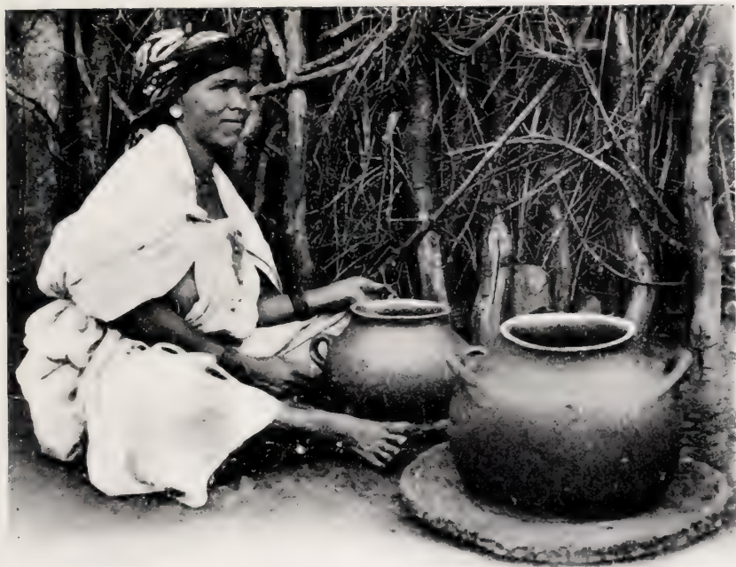
FIG. 89.—Native Kabyle woman of Algeria making earthenware without the aid of a potter's wheel. The vessel rests on a slab which she turns slowly round with her foot. Reproduced from the Revue d'Ethnographie , December 1911, by permission of M. A. Van Gennep.
